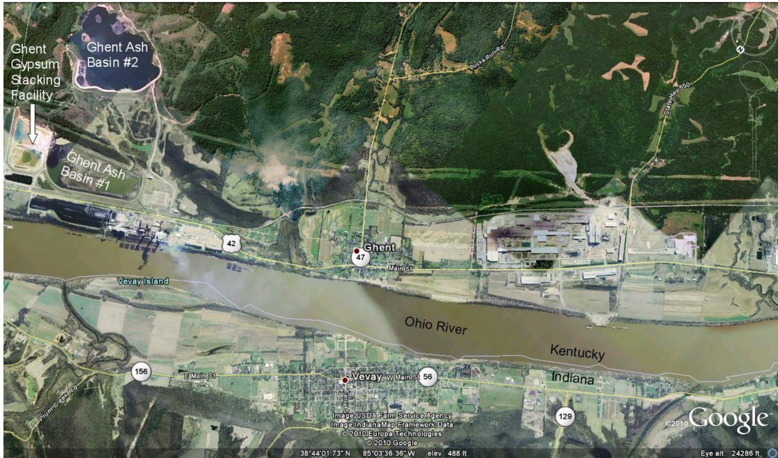
Ghent Ash Basins and Gypsum Stacking Facility: Located in Kentucky, all three of these facilities are rated “high-hazard” by EPA, with ash basin #2 reaching a height of 227 feet. 234 The nearby towns of Ghent, KY and Vevay, IN are only 1-2 miles away, 235 with many schools and churches arranged along the Ohio River. 236 Furthermore, the unlined 237 impoundments contain some of the highest levels of lead, nickel, and thallium in the nation. 238
